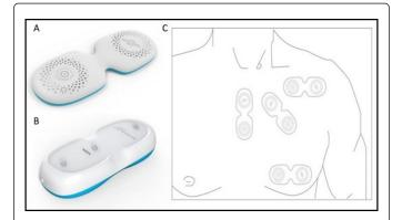
**Figure 1:** The Smartpatch II System, it contains a main structure for monitoring (A) as well as a base for recharging (B) and can be adhered on plain parts of the precordial area (C).
