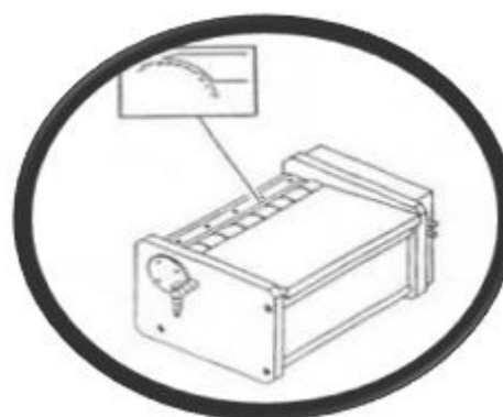
Figure 14. Fish de-skinning machine.
