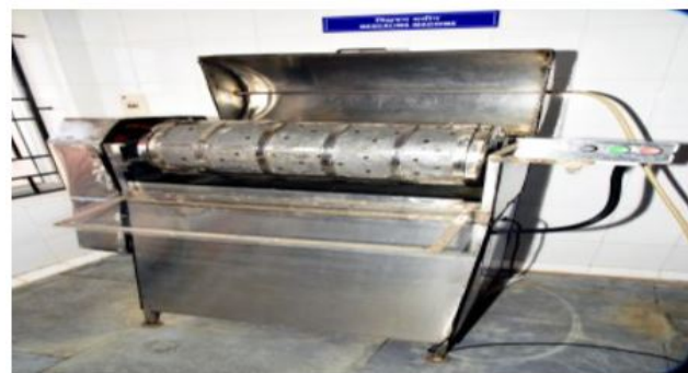
Figure 6. Fish de-scaling machine with variable drum speed.
