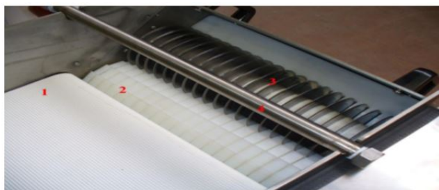
Figure 5. Working Instruction of drum and belt machine. (1) Conveyor belts; (2) Counter roller; (3) Blade unit; (4) Washing and cleaning systems.
