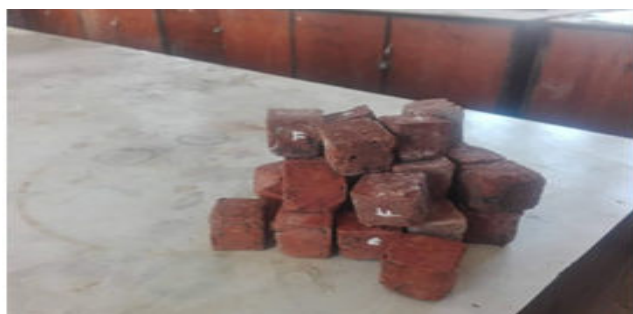
Figure 8. Prepared geopolymer cubes.
