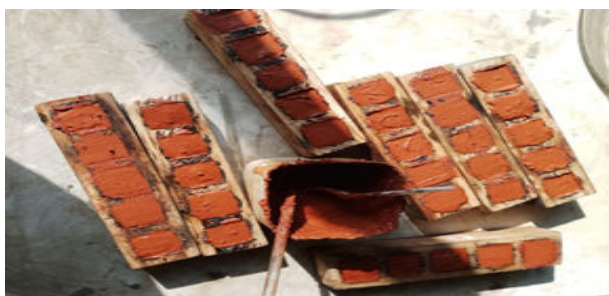
Figure 7. Preparation of geopolymer cubes.
