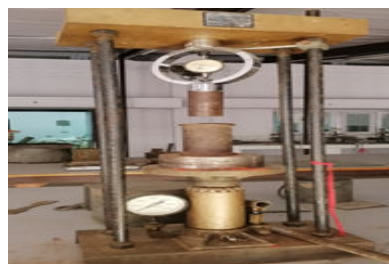
Figure 10. California bearing ratio machine.
