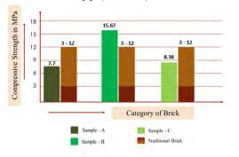
Figure 13. Comparison of compressive strength of developed and traditional brick
