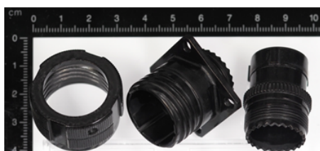
Figure 21. Sol-gel coating on Amphenol Socapex's connectors by dip-coating process
