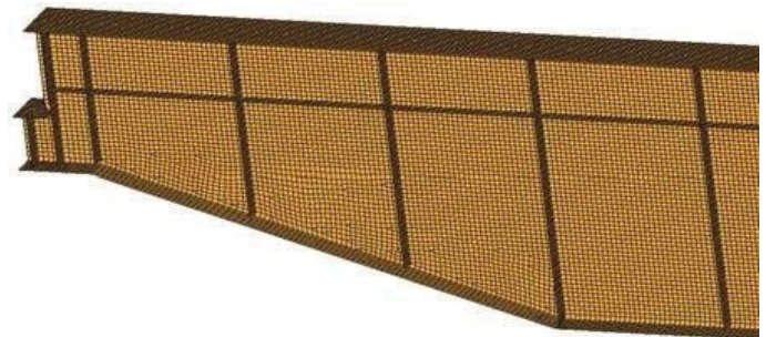
Figure 4. Meshing of crane girder.
