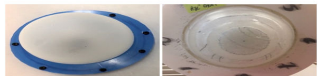
Figure 5. Deformation of elastomer-only (left) and elastomeric-fiber matrix (right) under Low Air Pressurization (3-15psi).
