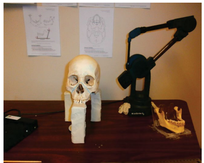
Figure 1. Tri-column clay stands with skull secured on top in close proximity to MicroScribe positioned in the homing position and mandible secured on a piece of plexiglass.
