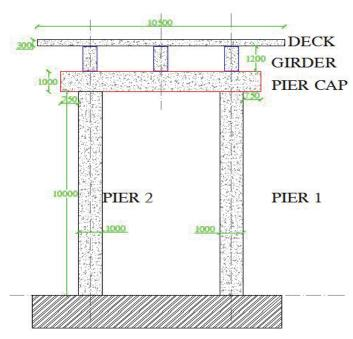
Figure 3. Typical cross-section of bridge.
