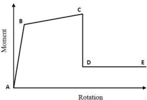
Figure 4. Moment-rotation curve idealized for RCC elements.
