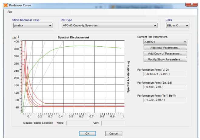
Figure 6. Capacity curve of the bridge NWBR S30M by CSM.
