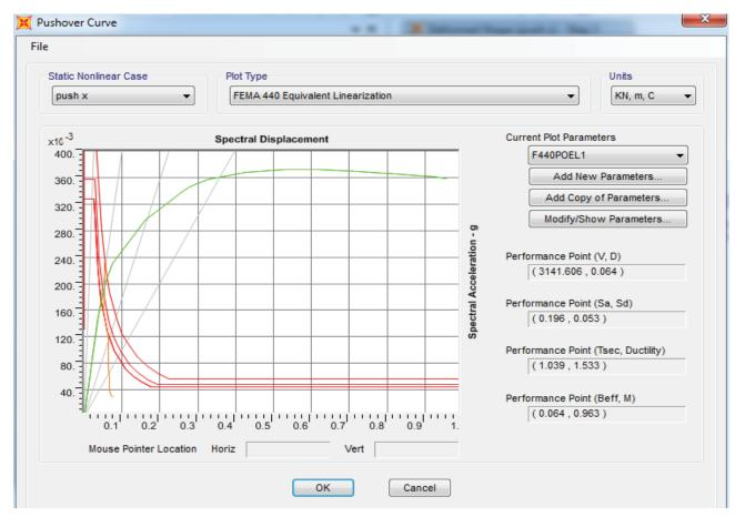
Figure 7. Capacity curve of the bridge NWBR S30M by ELM.
