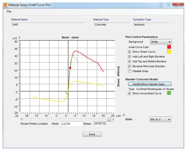
Figure 1. Stress-strain characteristics plot for M-40 grade of concrete as per Modified Mander's model.
