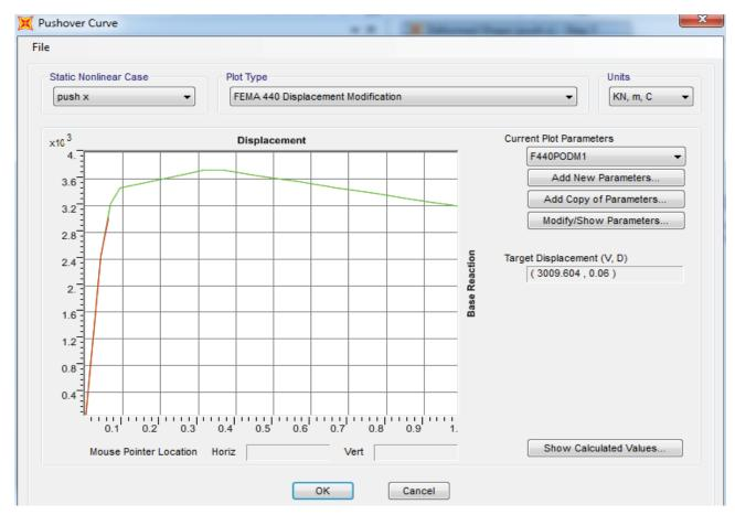
Figure 8. Capacity curve of the bridge NWBR S30M by DMM.
