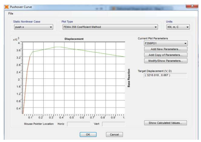
Figure 5. Capacity curve of the bridge NWBR S30M by DCM.
