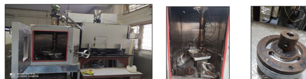
Figure 8. a) Centrifugal melt spinning setup, b) Spinneret setup with heater and c) Spinneret.
