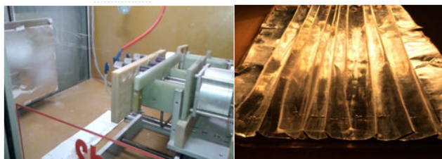
Figure 9. Electrospinning setup syringe pump with needle; zigzag aluminum collector resp.
