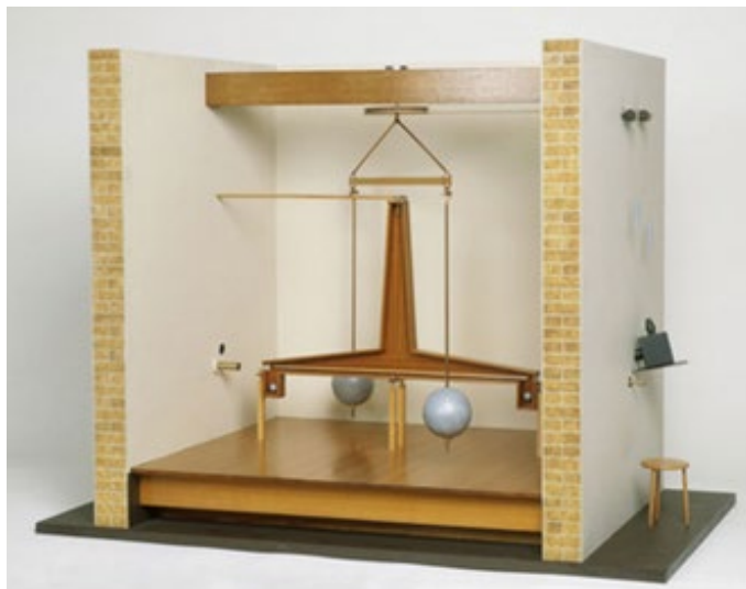
Figure 5. Model of the torsion balance Henry Cavendish, with which the gravitational attraction between laboratory bodies his first measured [Science Museum/Science & Society Picture Library].
