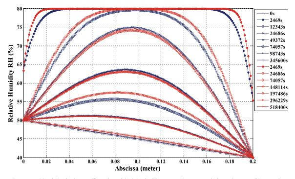
Figure 3. Spatial evolution of moisture at different times of simulation, for different pores sizes: 0.003 nm (red curves), 0.001 nm (blue curves).
