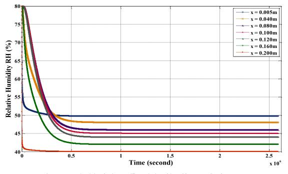
Figure 4. Temporal evolution of moisture at different abscissa of the wall for a pore radius of 0.001 nm.
