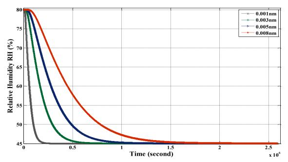
Figure 5. Temporal evolution of moisture in the middle of the wall, for different pores radius, 0.001 nm (black curve), 0.003 nm (green curve), 0.005 nm (blue curve) and 0.008 nm (red curve).
