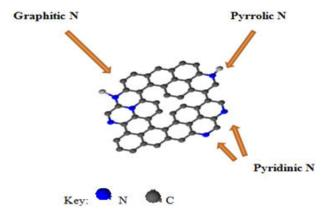
Figure 2. Doping position of N on graphen.
