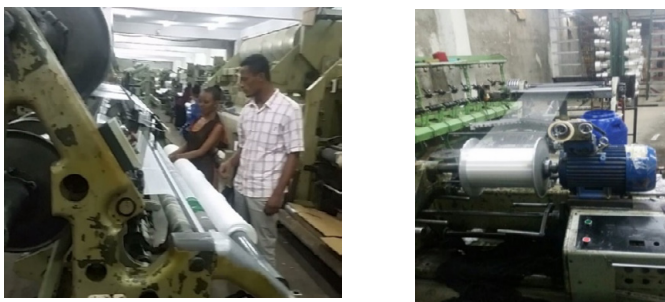
Figure 1. Sample preparation using Raschel machine.
