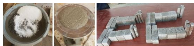
Figure 2. a) Chopped EPSw before the mixing b) Flow table test c) Cubic, prism, and cylinder specimens.
