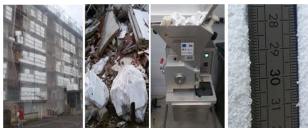
Figure 1. a) Huge quantity of EPS used for external insulation b) Collection of EPSw from the destructive building site c) Universal cutting mill d) Size of chopped EPSw.
