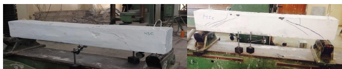
Figure 4. Crack patterns and failure mode of solid beam (Br-0) and bubbled beam (Br-16).
