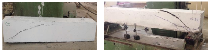
Figure 3. Crack patterns and failure mode of solid beam (Bn-0) and bubbled beam (Bn-16).
