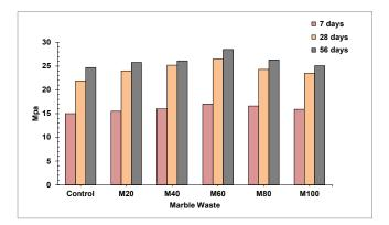
Figure 9. Split tensile strength results.
