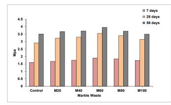
Figure 11. Flexure strength results.
