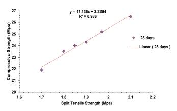
Figure 10. Co - relation between compressive and split tensile strength.
