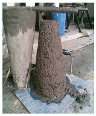
Figure 4. Slump test.
