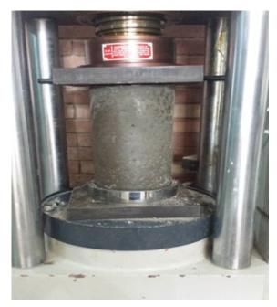
Figure 6. Compressive strength test.
