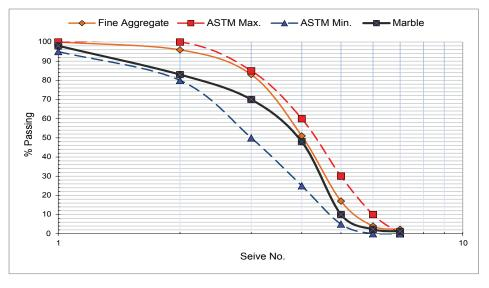
Figure 1. Gradation curve of marble and fine aggregate.
