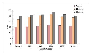
Figure 7. Compressive strength results.
