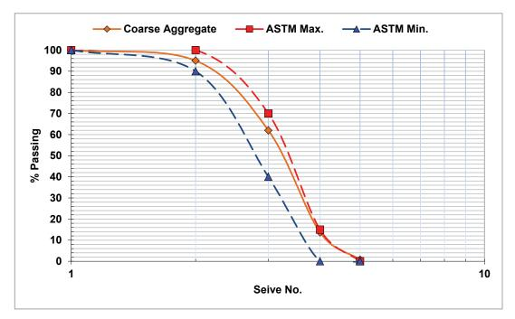
Figure 2. Gradation curve coarse aggregate.
