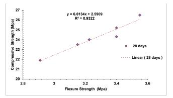
Figure 12. Co - relation between compressive and flexure strength.
