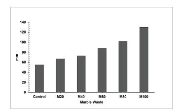
Figure 5. Slump test results.
