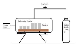
Figure 6. Carbonation chamber model.
