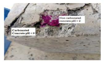
Figure 12. Degree of carbonation.
