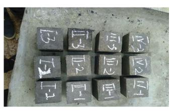
Figure 9. Cement mortar cube specimen.
