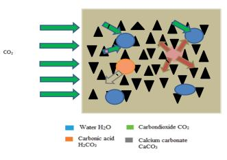
Figure 2. Carbonation in concrete.
