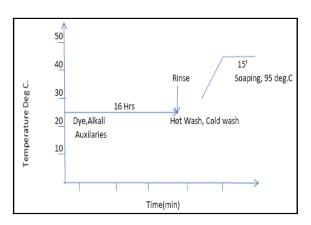
Figure 2. Process flow of pad batch dyeing.
