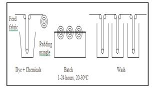
Figure 1. Pad-batch method.
