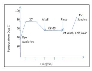
Figure 3. Process flow of Novacron Brilliant Blue H-GR.
