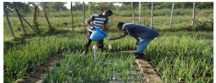
Figure 1. Water application by using graduate cylinder to the Lysimeters and surrounded fields.
