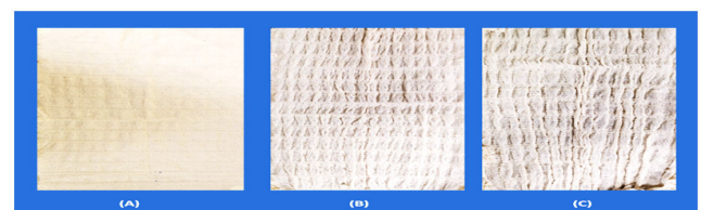
Figure 7. Image analysis of fabric having different counts A) 60/2 ss; B) 20 s; C)16 s.
