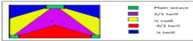
Figure 3. Unit cell of double arrow geometry along with deformation zones.
