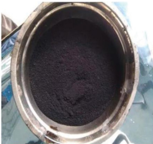
Figure 2: Crumb rubber modifier used in this study.
