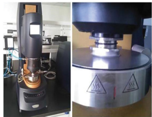
Figure 5: DSR experimental setup and sample sandwiched between two plates.
