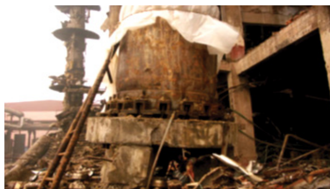
Figure 1. Urea synthesis reactor exploded in a fertilizer plant in Pingyin County.
