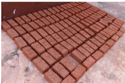
Figure 5: Moulded blocks ready for curing.
