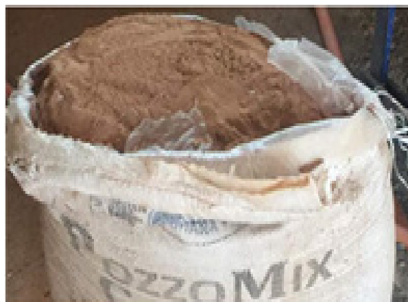
Figure 3: Bag of pozzolana.
