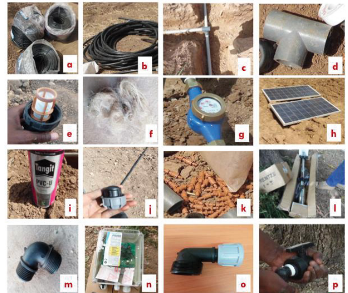
Figure 2. Technical equipment used for the implementation of the installations of the drip irrigation system: 2a) Gutter tube 2b) PE tube 2c) PVC tube inside the trench before burring 2d) T-PVC, 2e) Strainer filter 2f) Yarn doll 2g) Flowmeter 2h) Solar panels 2i) Glue box 2j) Stopper 2k) Junctions 2l) Pum 2m) Male elbow 2n) Regulator 2o) Female elbow 2p) Valve.
