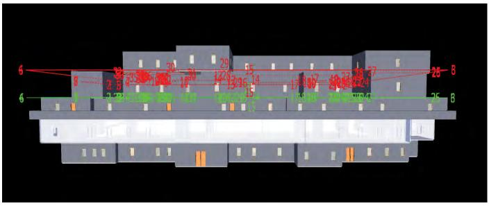
Figure 17. Shows the construction of the third floor and shows green faded components on the fourth floor that are in queue for construction after the completion of the current. In such a way the entire construction process can be visualized virtually from start to finish and time schedules can be revised for improvements that help in optimized and effective usage of resources available for construction.
