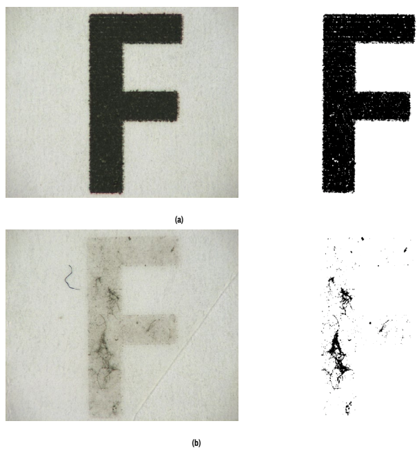
Figure 6. Original image of the old inkjet-printed characters exfoliated with adhesive tape. (a) Binarized image of the old inkjet-printed characters before adhesive-tape exfoliation and (b) Binarized image of the ink transcribed to the tape through adhesive-tape exfoliation.
