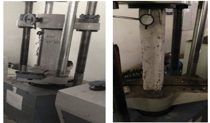
Figure 2. Testing of short column.
