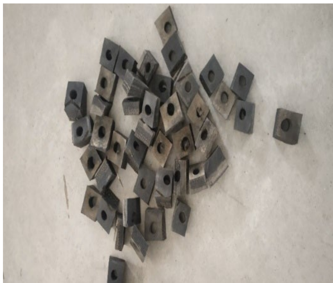
Figure 1. 10 mm diameter hole on the surface of the reshaped tyre rubber.
