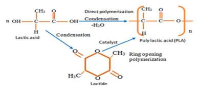
Figure 2. PLA polymerization [46].
