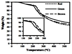
Figure 4. TGA (Thermogravimetric analysis) curve of red, green and brown algae flakes of 200-400 µm [73].
