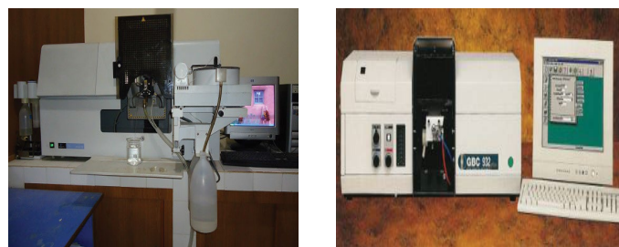
Figure 4. Atomic Absorption Spectrophotometer (A) AAS 700 and (B) GBC 932 Plus.
