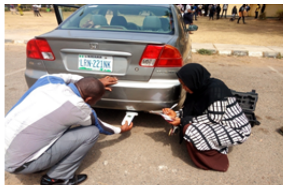
Figure 1. Experiment of vehicle gas emission of Carbon monoxide (co) using gas analyzer monitor aeroqual series 500 with carbon monoxide sensor head.
