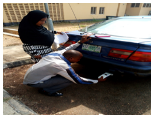
Figure 2. Experiment of vehicle gas emission of Nitrogen Oxide (NO 2 ) using gas analyzer monitor aeroqual series 500 with nitrogen oxide sensor head.
