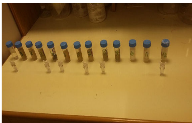
Figure 10. Samples and cells for testing zeta potential.
