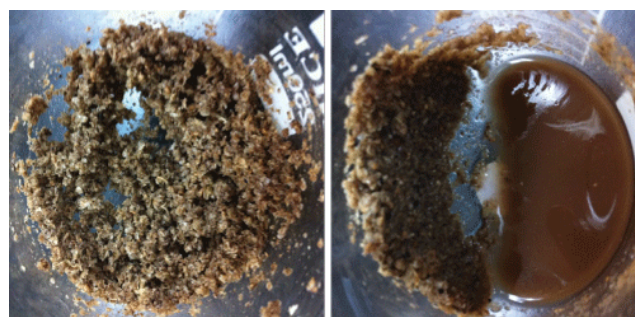
Figure 1: Culture flask containing agricultural extract as the carbon source for the production of xylanase by B. subtilis in SsF (left). Sterile distilled water was added into the carbon source to extract the sample from culture flask in SsF for analysis (right).
