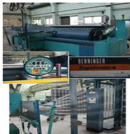
Figure 2: Benninger warping machine showed the attached applied tension equipment.
