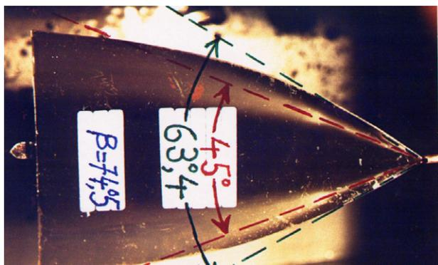
Figure 3: View n° 3 – View of the upper surface:  $\beta=74.5^\circ$   $i=40^\circ$   $\alpha_1=45^\circ$   $\alpha_2=63.4^\circ$ .
