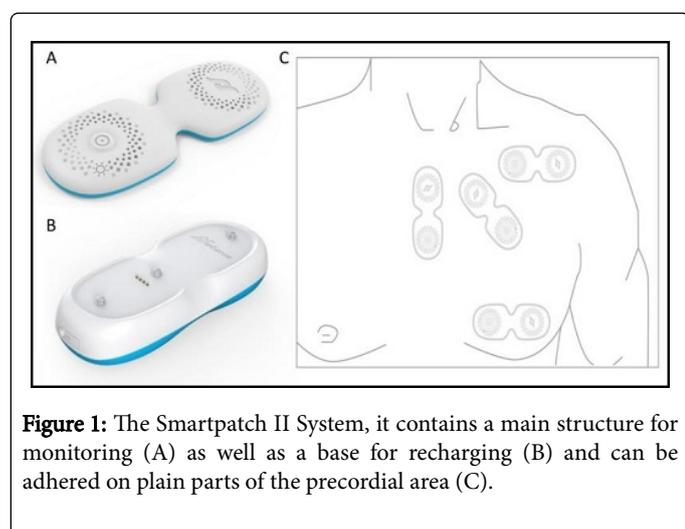
**Figure 1:** The Smartpatch II System, it contains a main structure for monitoring (A) as well as a base for recharging (B) and can be adhered on plain parts of the precordial area (C).
