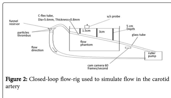
**Figure 2:** Closed-loop flow-rig used to simulate flow in the carotid artery
