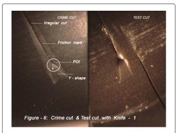
Figure 6: Crime cut and test cut with knife.
