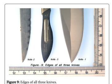
The comparison made between the puncture marks made by the above said three knives, whose close-up blade edge view is given in Figure 9, on the P.V. tubing showed the difference in puncture made by each knife. The comparison made showed that the knife in the Figure 1 had caused the puncture mark on the tubing shown in the Figure 4 and its comparison shown in the Figure 6.
