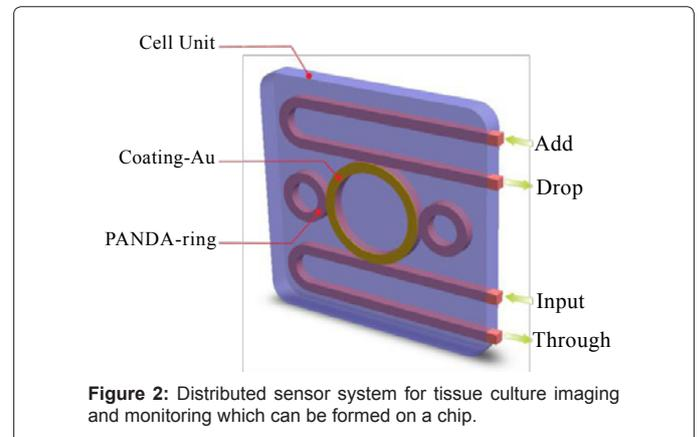
Figure 2: Distributed sensor system for tissue culture imaging and monitoring which can be formed on a chip.
