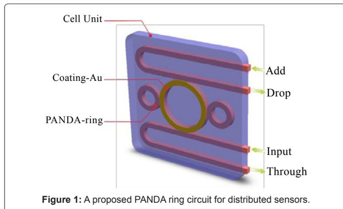
Figure 1: A proposed PANDA ring circuit for distributed sensors.
