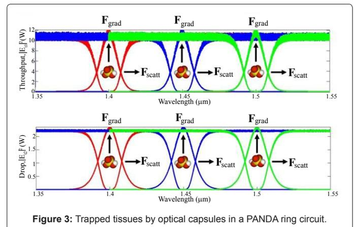
Figure 3: Trapped tissues by optical capsules in a PANDA ring circuit.
