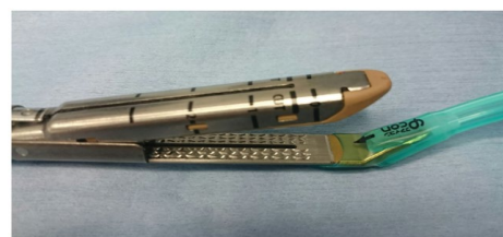
Figure 3: An anvil was placed onto the mounting head of the silicone tube.
