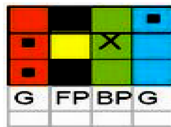
Figure 2: The weave repeat of the terry fabric (Basic 3-pick terry weave in 2:2 warp order [42].
