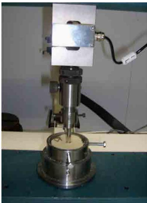
Figure 2: Implant / Synthetic Bone Construct in Position for Pushout Testing.
