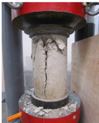
Figure 2: Compression strength test in concrete.
