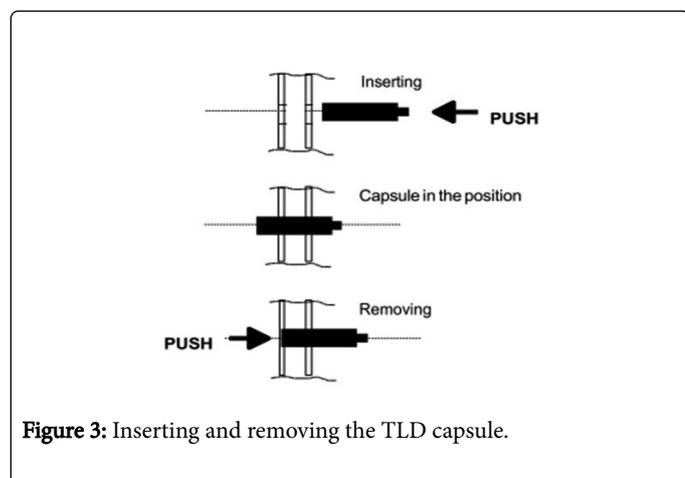
Figure 3: Inserting and removing the TLD capsule.
