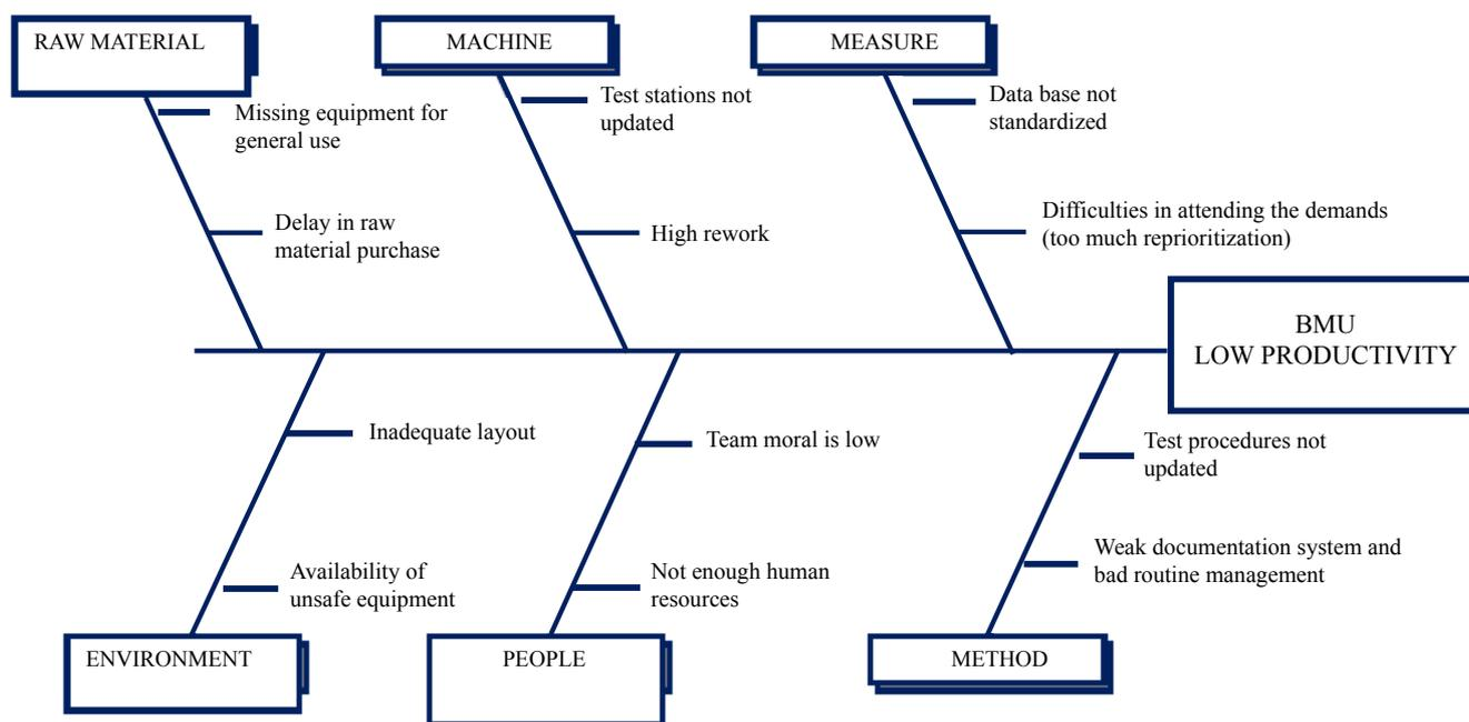
Figure 3: Diagram of the possible causes of low productivity in the analyzed area.
