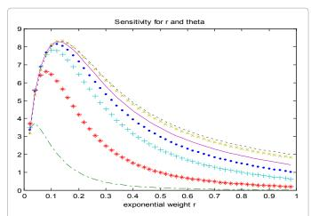
**Figure 3c:**  $S_{\rm rk}(\theta)$  for Sensitivity  $\eta_2$  of M-EWMA Chart for Dispersion Shift, k=10 Steady State (i=100).
