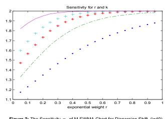
Figure 2: The Sensitivity  $\,\eta_2^{}$  of M-EWMA Chart for Dispersion Shift, (i=40). '•': k=5; '-.': k=10; '\*': k=15; '+': k=20; '--': k=30
