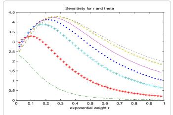
Figure 3b:  $\mathcal{S}_{\mbox{\tiny \it{fk}}}(\theta)$  for Sensitivity  $\,\eta_2\,$  of M-EWMA Chart for Dispersion Shift, k=5 Staring State (i=10).  $\text{`-.':} \theta = \text{-0.8}; \quad \text{`*':} \ \theta = \text{-0.5}; \ \text{`+':} \ \theta = \text{-0.2}; \quad \text{`-':} \ \theta = 0; \ \text{`--':} \ \theta = 0.2; \ \text{`x':} \ \theta = 0.5;$ '- -':*θ* =0.8;
