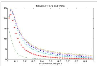
**Figure 3d:**  $S_{\kappa}(\theta)$  for Sensitivity  $\eta_2$  of M-EWMA Chart for Dispersion Shift, k=30 Steady State (i=100).
