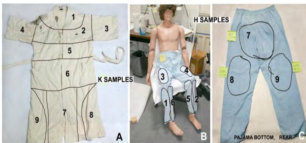
**Figure 7:** SEM sampler series H and K. Sixty dabs per sample. A: Sample regions of the bathrobe (samples K-1 through K-9). B: The front areas of the pajama bottom (Samples H-1 through H-6). C: The back of the pajama bottom showing the SEM tape lift area H-7 (buttocks), H-8 (left rear thigh) and H-9 (right rear thigh).
