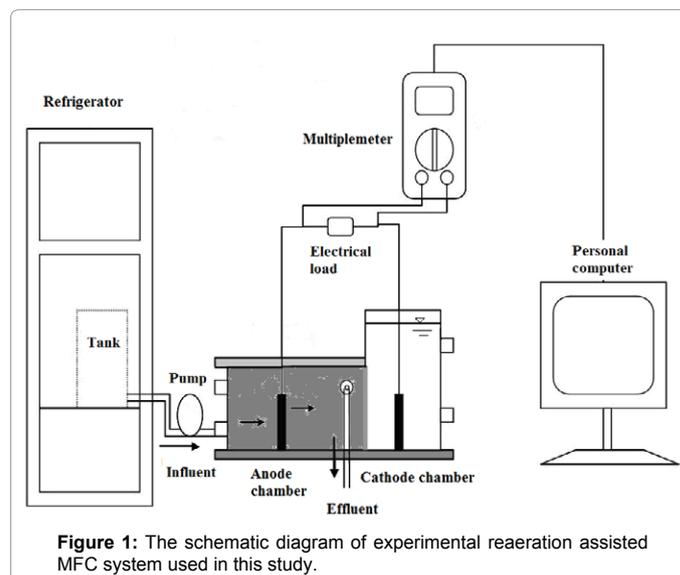
Figure 1: The schematic diagram of experimental reaeration assisted MFC system used in this study.
