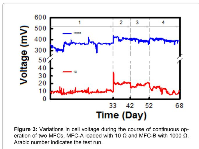
Figure 3: Variations in cell voltage during the course of continuous operation of two MFCs, MFC-A loaded with 10  $\Omega$  and MFC-B with 1000  $\Omega$ . Arabic number indicates the test run.
