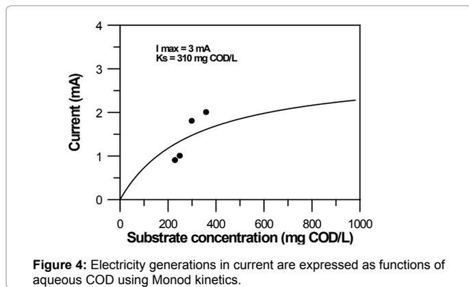
**Figure 4:** Electricity generations in current are expressed as functions of aqueous COD using Monod kinetics.
