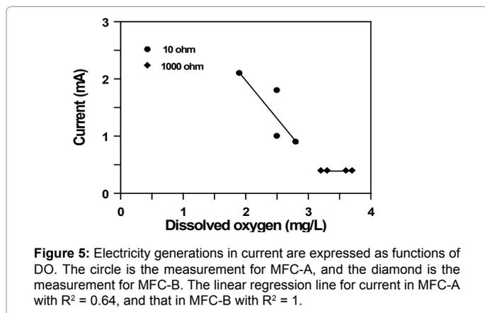
**Figure 5:** Electricity generations in current are expressed as functions of DO. The circle is the measurement for MFC-A, and the diamond is the measurement for MFC-B. The linear regression line for current in MFC-A with R<sup>2</sup> = 0.64, and that in MFC-B with R<sup>2</sup> = 1.
