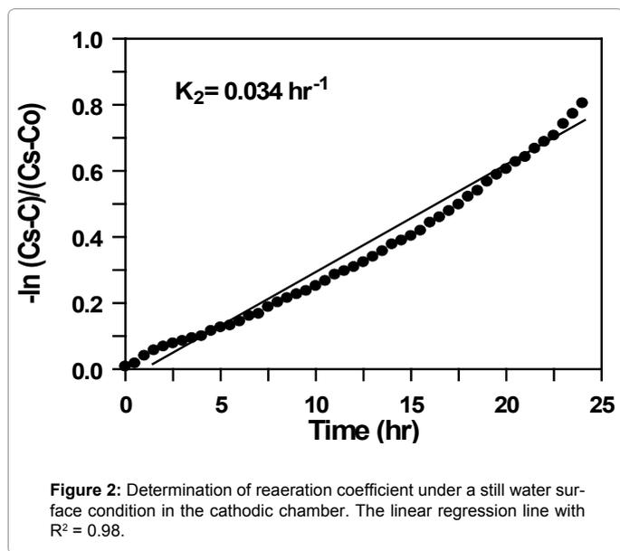
Figure 2: Determination of reaeration coefficient under a still water surface condition in the cathodic chamber. The linear regression line with  $R^2 = 0.98$ .
