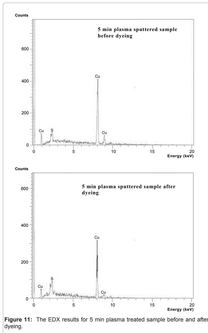
Figure 11: The EDX results for 5 min plasma treated sample before and after dyeing.
