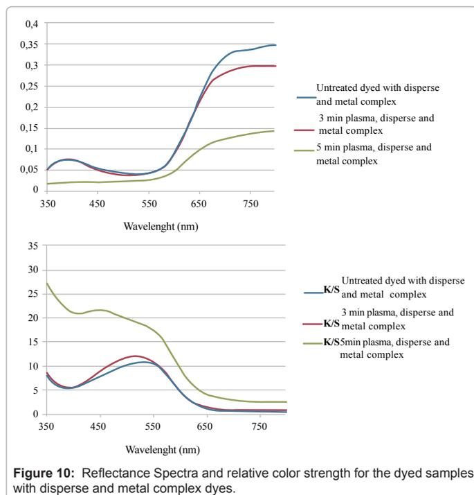
Figure 10: Reflectance Spectra and relative color strength for the dyed samples with disperse and metal complex dyes.
