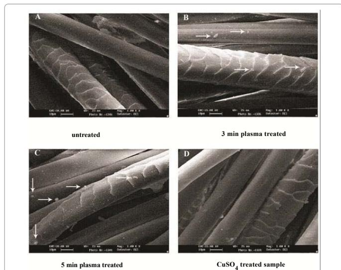
**Figure 2:** The SEM images of mordanted and plasma treated samples, A-Untreated sample, B-3 min plasma treated sample, C-5 min plasma treated sample, D-CuSO<sub>4</sub> (mordant) treated sample.
