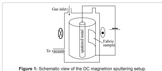
Figure 1: Schematic view of the DC magnetron sputtering setup.
