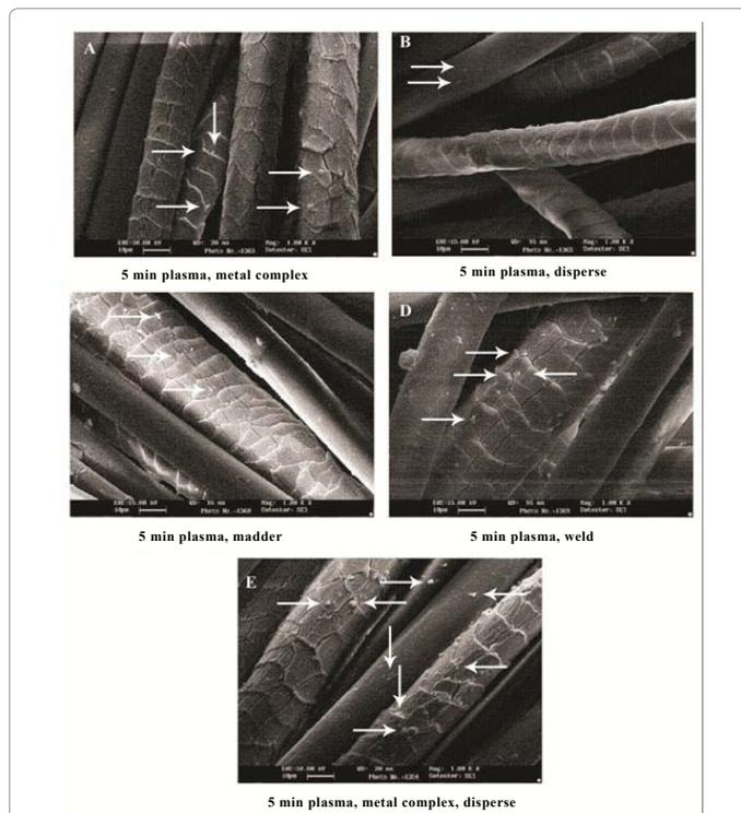
**Figure 5:** The SEM images of plasma treated samples for 5 min after dyeing with different classes of dyestuffs, A-5min plasma treated dyed sample with metal complex dye, B-5min plasma treated dyed sample with disperse dye, C-5min plasma treated dyed sample with madder dye, D-5min plasma treated dyed sample with weld dye, E- 5min plasma treated dyed sample with metal complex and disperse dyes.
