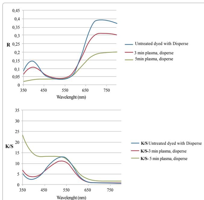
Figure 9: Reflectance Spectra and relative color strength for the dyed samples with disperse dye.
