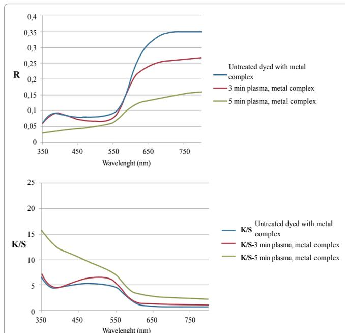
Figure 8: Reflectance Spectra and relative color strength for the dyed samples with metal complex dye.
