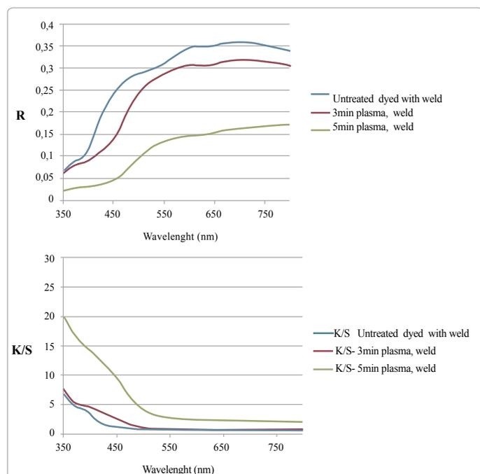
Figure 7: Reflectance Spectra and relative color strength for the dyed samples with weld.
