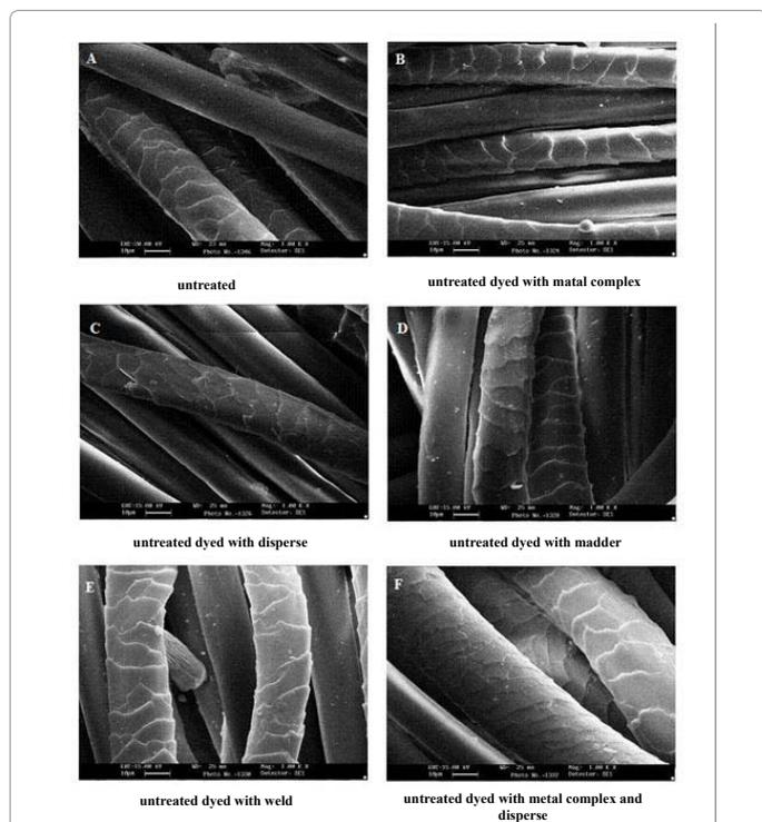
**Figure 3:** The SEM images of dyed untreated samples with different classes of dyestuffs, A-Untreated sample, B- Untreated dyed sample with metal complex dye , C-Untreated dyed sample disperse dye, D-Untreated dyed sample with madder dye, E-Untreated dyed sample with weld dye, F-Untreated dyed sample with metal complex and disperse dyes.
