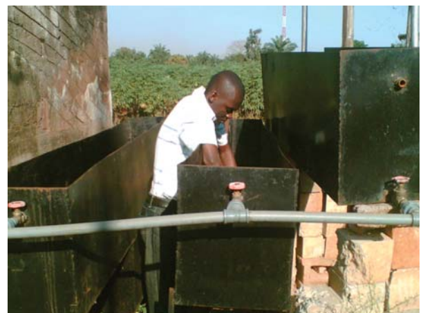
Figure 3: Addition of Common Salt for Tracer Studies.
