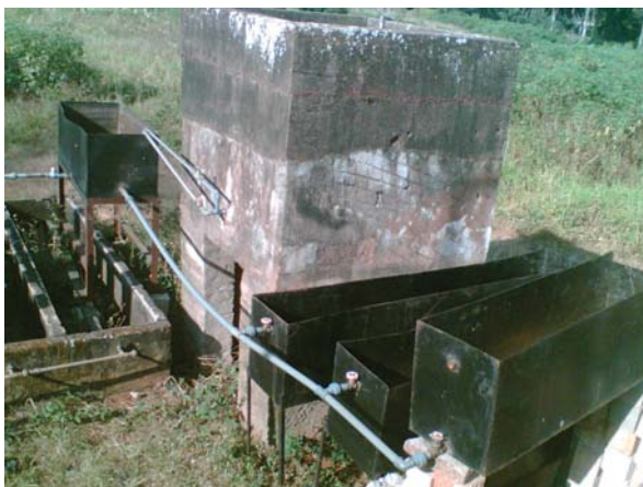
Figure 1: Experimental Setup. The overhead storage tank (1.2m×1.5m×1.5m) was usually filled intermittently with sewage from the University of Nigeria, Nsukka, Nigeria facultative WSP through an underground pipe with a pump. The sewage storage tank (1.2m×0.5m×0.5m) gets its supply from the overhead storage by gravity flow through a pipe connecting both. Both tanks were usually filled to supply the three ponds with sewage wastewater. The samples were collected at an interval of twice per week from the three ponds for ten weeks. Samples were collected from one pond at a time. For Pond 0, samples (0a and 0b) were collected at both the inlet and outlet. The wastewater flows into the experimental ponds through an inlet (19mm diameter) pipe. The wastewater flows out of the pond through a slit. For Pond 1 and Pond 2, five samples each were collected at intervals of 160mm at different points along the channels. These points corresponded to 1a, 1b, 1c, 1d, 1e, 2a, 2b, 2c, 2d and 2e for Pond 1 and Pond 2 respectively. Thereafter, samples collected from the three ponds were taken for laboratory analysis to determine the concentration of BOD, COD, total Coli form and Dissolved Oxygen. Date of collection of sample was recorded for the duration of the research.
